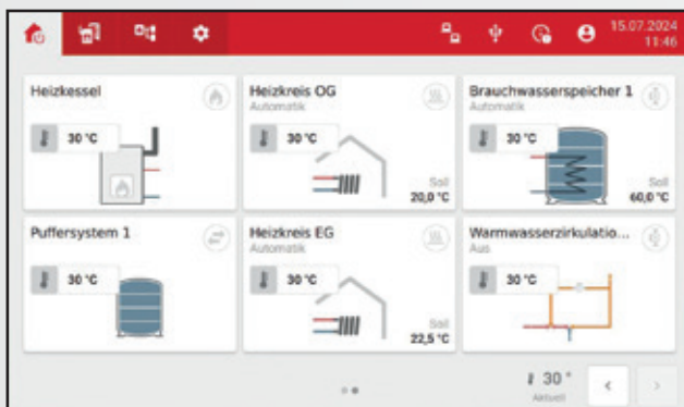
Overview of the installed components in a tile display
